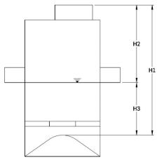
H1: distance between the top of the cast iron frame and the top of sediments.
