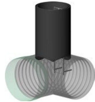
MANHOLE CATCH BASIN CHIMNEY TYPE WITH SMOOTH EXTERIOR WALL
