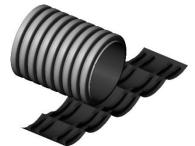
Insert the split coupler under one of the 2 pipes on the central part.
