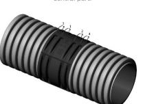
Insert and secure the cable ties without tightening them.
